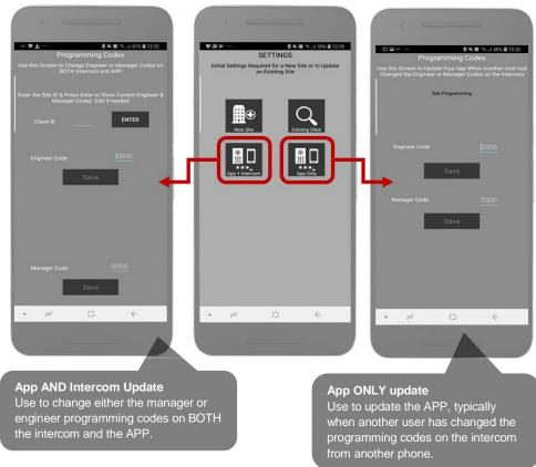
Note: This app sends SMS programming strings to the intercom as shown and it should reply with OK message. On iphones, due to restrictions by Apple, you must confirm the SMS as shown. Android devices will auto send the SMS in the background.
